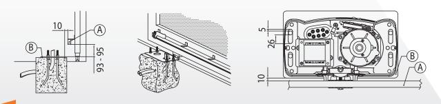
A = Rack B = Fastening plate (thickness 3mm)
