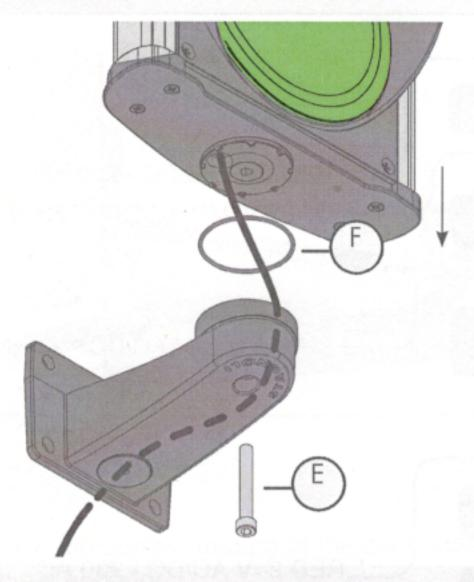
When the bottom cover is closed, fasten the body to the lower bracked previously fixed (Page 9), by means of the special self-tapping screw [E], paying attention to the repositioning of the OR ring [F]
