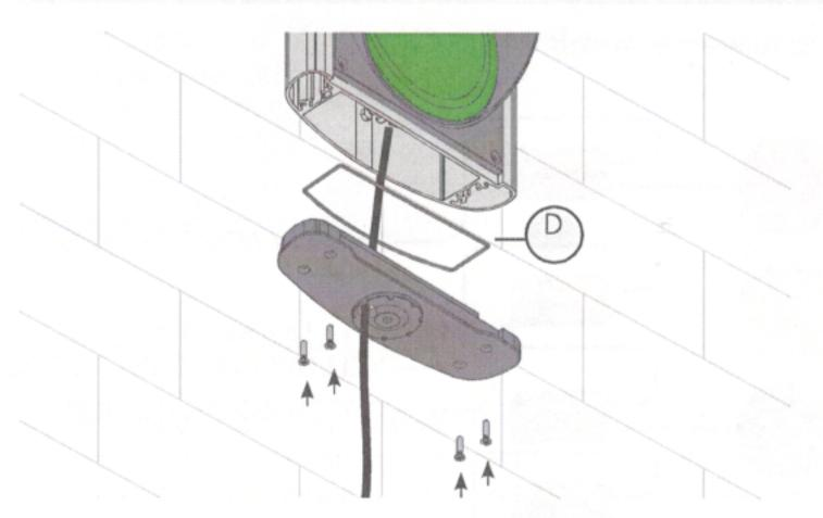
When the wiring is finished, close the cover ensuring that the OR ring is repositioned [D]
