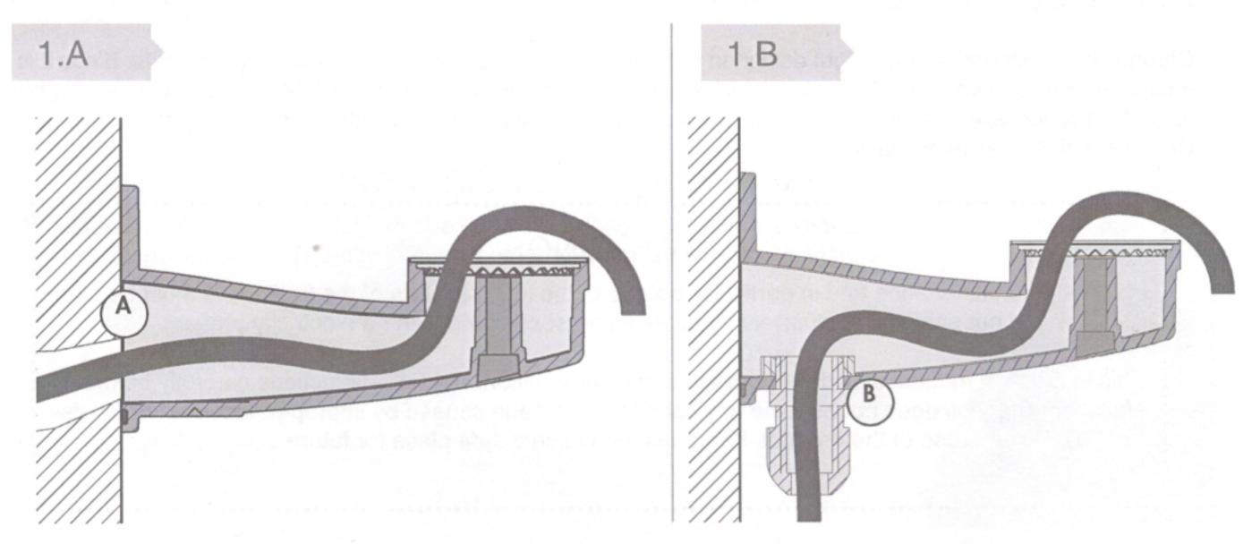
Once the correct routing of the cable has been set, fix the bracket to the wall using the suitable screws and screw anchors.
