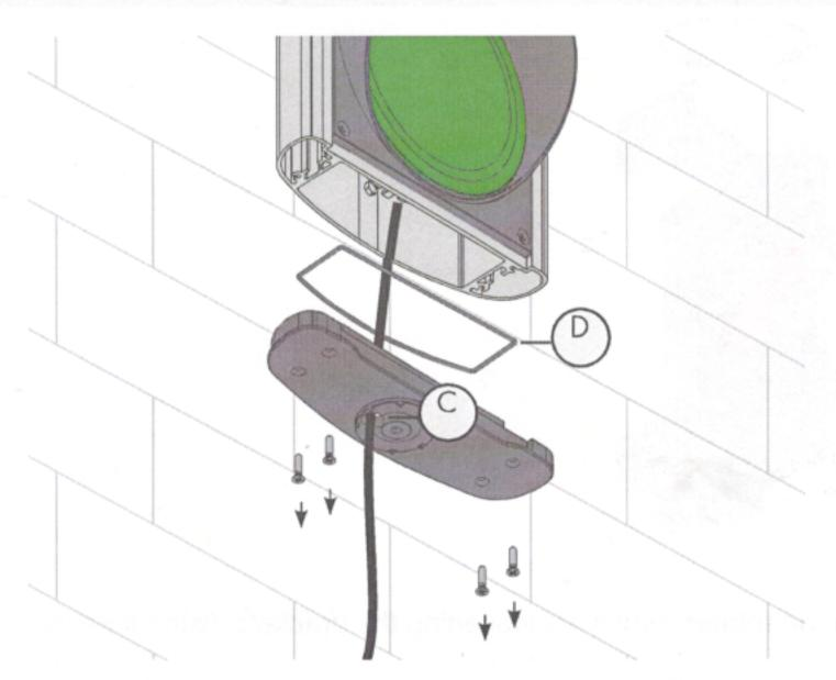
Open the bottom cover by unscrewing the 4 Phillips head screws placed on the bottom.
