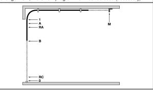
These manoeuvres are carried out at low speed. If the door is in the closing position, it must be positioned manually at about 50 cm from the ground, using the emergency system (see the motor instruction manual) in order to prevent, if the rotation is reversed, the track ropes from coming out of their housing (sectional doors) or the excessive winding of the shutters (rolling shutters).
