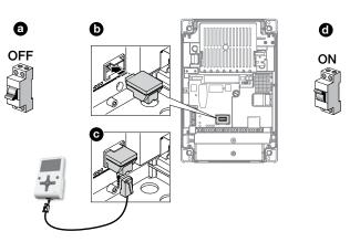
A CAUTION! - If the functions of Table 3 are programmed with the Oview programming unit, it is necessary to set the dip switches to OFF.
